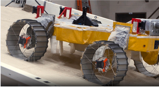
Fig. 28. MGRU3 climbing a “tilt bed” in NASA’s Glenn Research Center testing facility [95].
