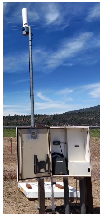
Fig. 3: Installed Sensor Node showing the Keysight N6850A Antenna, the pre-amplifier box and the EMI enclosure inside the open field cabinet
