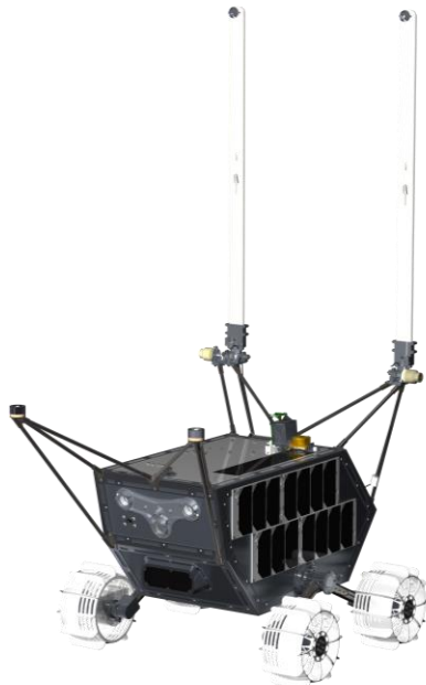
Figure 2. Lunar Outpost rover with Nokia UE and deployed rover antennas.
