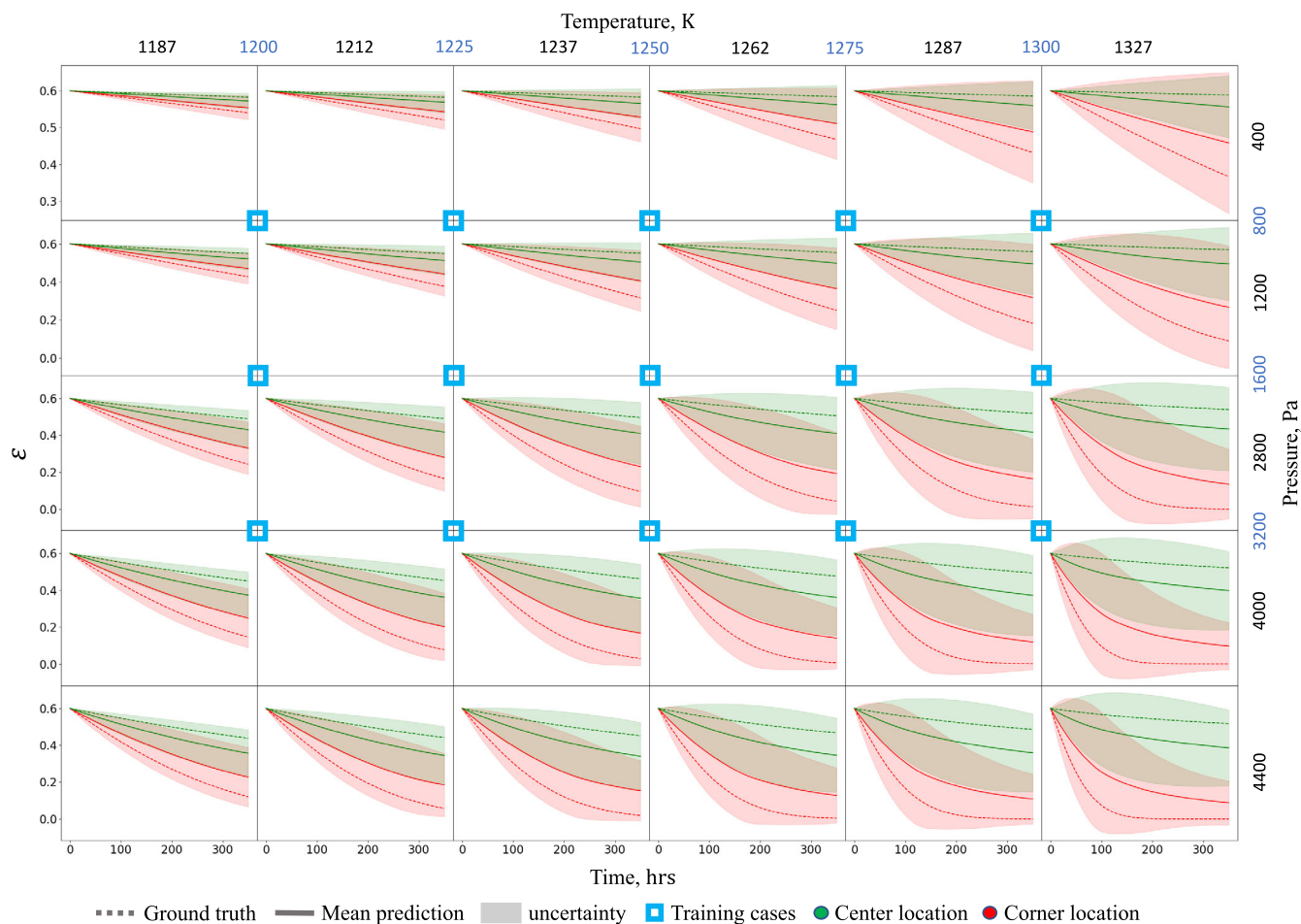
Fig. 9 | PiNDiff predictions on porosity with uncertainty for unseen partial pressure and temperature. The model is trained on synthetic total mass data.
