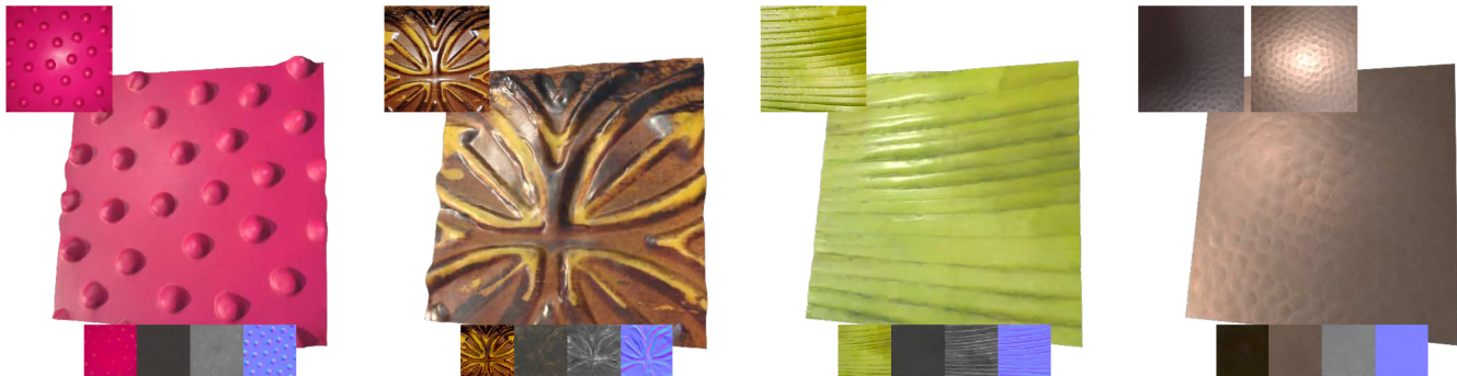
Figure 1: SVBRDF diffusion estimates visualized with integrated normal maps and global illumination for four different spatially varying materials captured by: a colocated flash photograph (1st and 2nd), a photograph captured under uncontrolled natural lighting (3rd), and a flash/no-flash image pair (4th).
