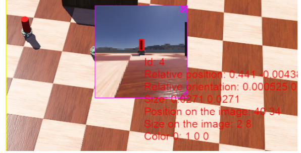
Figure 3: Webots has built-in object recognition that provides relative position, relative orientation, size, position on the image, size on the image, and color.
