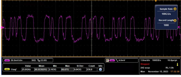
FIGURE 16. The portion of the target qubit analog waveform recorded on real-time scope (corresponding to 1551 nm wavelength).
