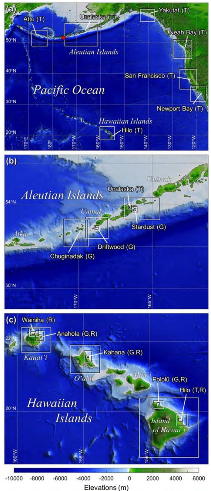
Fig. 2. Location map for tsunami observations and computational grids. (a) Level-1 and 2 grids for North Pacific and regional computations with epicenter (red star) and tide-gauge (T) locations. (b) Level-2 to 5 grids for eastern Aleutian Islands with additional geologic (G) record locations. (c) Level-2 to 5 grids for major Hawaiian Islands with additional runup (R) record locations.
