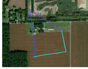
(b) Flight replay showed that the sUAS flew north at increasing altitude after the geofence breach.
