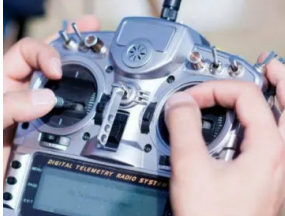
(c) The RPIC must position the throttle correctly in case in-flight problems require human control.
