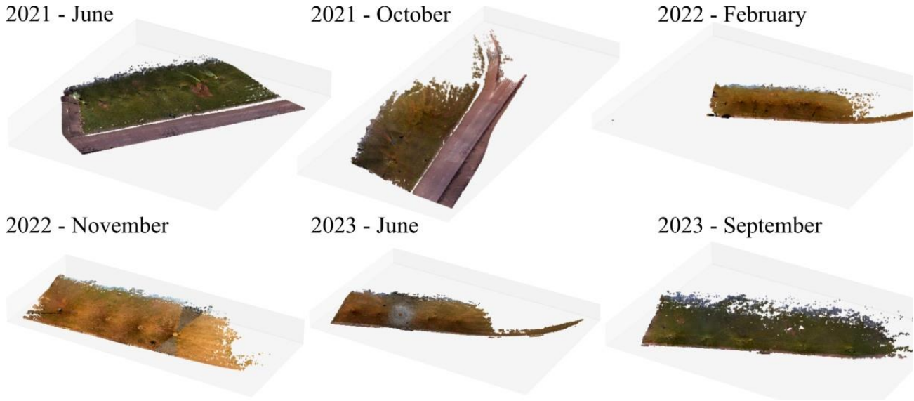
Figure 3: LiDAR point cloud surface topography of the monitored embankment for the size scans from 2021-2023.
