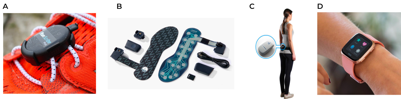
Figure 1: The 4 example wearables that we presented to PTs during Activity 2, these were: (A) a wearable used by runners that is attached to shoelaces; (B) a pressure-sensitive system for insoles; (C) a clinical sensor for balance and gait worn on a belt around the waist; and (D) a consumer smartwatch.
