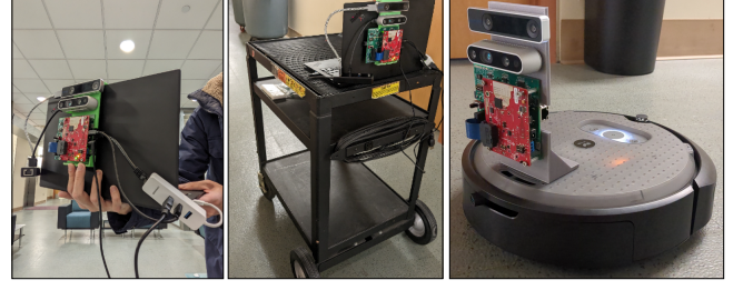
FIGURE 10: Left. Moving sensors by hand. Center. Sensors mounted on a cart. Right. Sensors mounted on robot.
