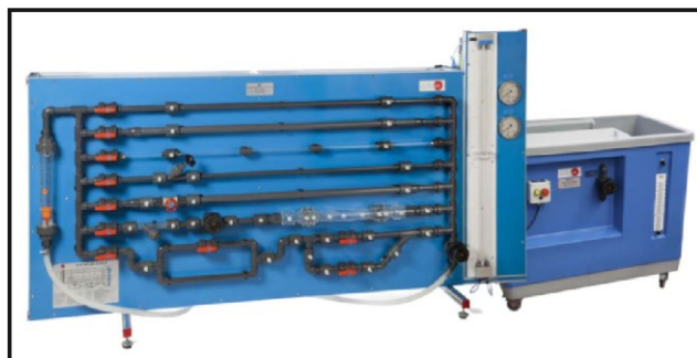
Figure 2. Edibon AFT-B Fluid Flow in Pipes equipment that is used at PVAMU Chemical Engineering Laboratory.
