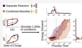
reactor size and cost. Comparing the minimum energy demand and process time of this combined reactor to those of the separated configuration, we found that the combined absorber can reduce the energy demand by up to 67% but doing so can also increase the process time by several orders of magnitude. In contrast, optimizing the solution chemistry could benefit both the energy demand and process time simultaneously.
