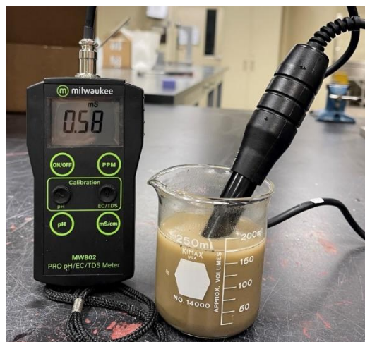
Figure 4. The conductive meter used to measure the salinity in the soil and a beaker with soil-water suspension.
