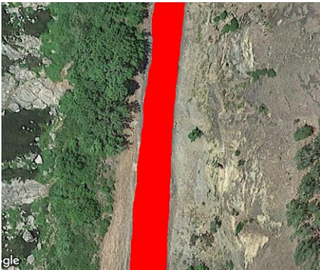
Figure 6. The segmentation from YOLOv8 custom dataset model for road in Figure 4
