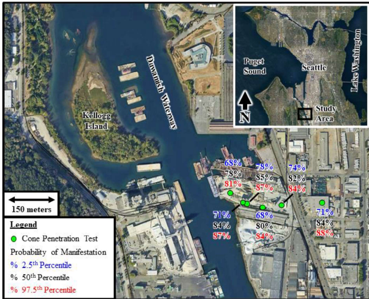
Figure 4. Probabilities of liquefaction surface manifestation expected in 30 different ground motion simulations; the 2.5 th , 50 th , and 97.5 th percentiles of the probability of manifestation, considering all 30 simulations, are mapped at each CPT site.
