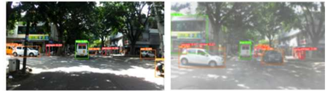
Figure 1. YOLOv5n [1] object detector fails to detect objects accurately due to foggy weather.
