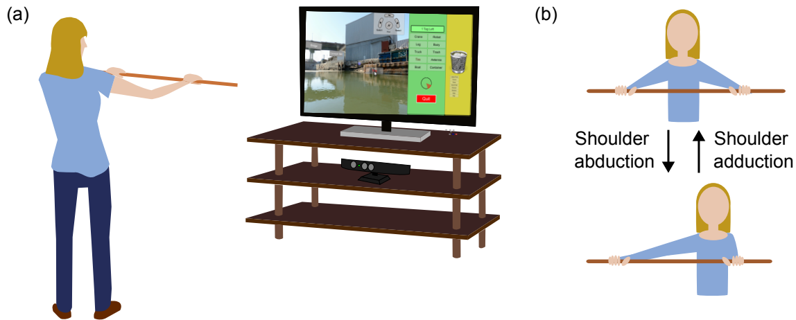
Figure 1. Experimental set-up of the telerehabilitation platform. The user holds a dowel and manipulates it with both hands to control an application that is launched on a monitor (a). A Kinect sensor is positioned below the monitor to record the user's movements. The present study focuses on machine learning of horizontal shoulder abduction/adduction (b).
