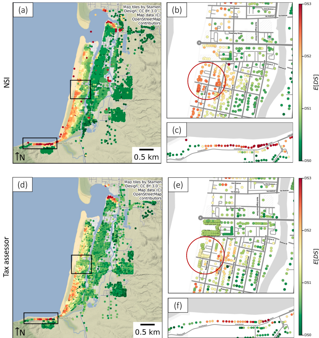
Fig. 7. Expected damage state of NSI (top row; panels a, b, and c) and tax assessor buildings (bottom row; panels d, e, and f) for the 500-yr recurrence interval.
