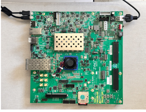
Fig. 2. Target Board (Xilinx's Zynq ZCU102)
