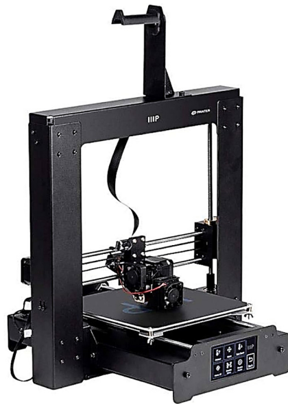
Figure 1. A Monoprice Maker Select Plus FDM printer which was modified and used for FKM and FFKM 3D printing.
