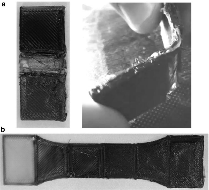
AU16 ▶ FIG. 8. Printed test applications: (a) living hinge, which used PLA for rigid portions and TPU for hinging portions, and (b) graduated tensile bar, which used white and black PLA. PLA; TPU, thermoplastic polyurethane.
