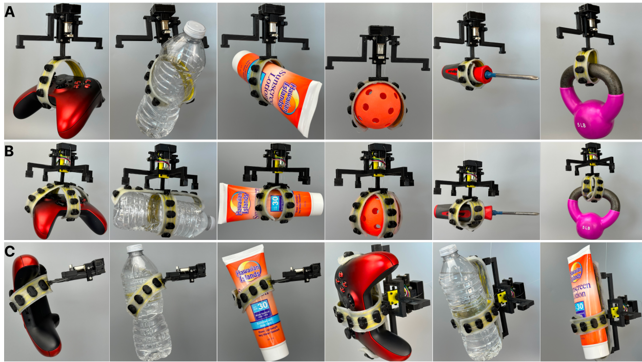
Fig. 7. Object grasping performance for both grippers in the horizontal axis where: (A) Horizontal grasping for the single-band gripper for (left to right) a video game controller, half-full plastic water bottle, full sunscreen bottle, wiffle ball, screwdriver, and 5 pound kettlebell. (B) Horizontal grasping for the cross-shaped gripper for the same objects as the single-band gripper; (C) Vertical grasping for both grippers with (left to right) a game controller, a full plastic water bottle, and a full sunscreen bottle.
