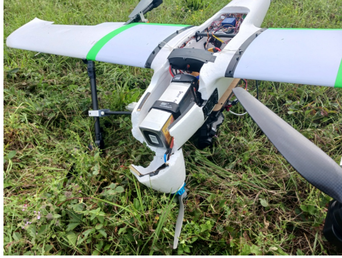
Fig. 9. Our VTOL drone crash-landed and broke its nose due to a real-life tug-of-war in which the autopilot initiated RTL, overriding the pilot's decision to land in QHOVER mode when a sudden drop in battery voltage occurred.
