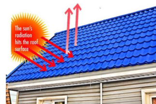
Figure 13. Schematic diagram of the solar radiation reflective coating roof.
