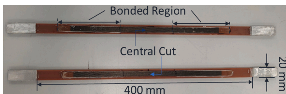
Fig. 10. Manufactured sensors attached to S-Glass/Epoxy substrate.
