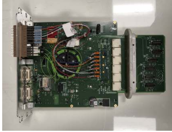
Figure 95. The pixel PortCard for Run 3; the small flange near the bottom acts as a feed-through for the board. The section below is housed inside the secondary vacuum volume of the pot.
