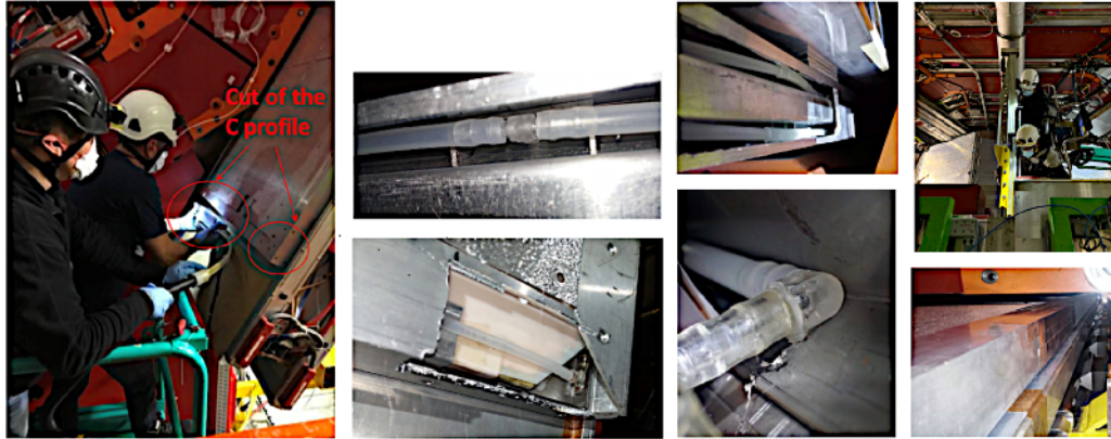
Figure 70. Photographs illustrating the gas-leak repair procedures. Left: scientists working on the repair procedure. Middle left: access to broken component. Middle right: repairing of components. Right: closing and validation.
