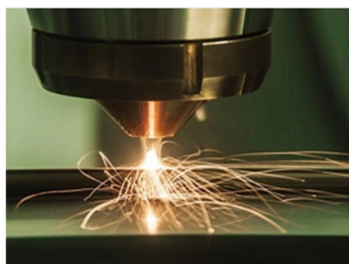
Figure 16. Image of laser powered DED process [107]. Copyright 2019, 3D natives.
