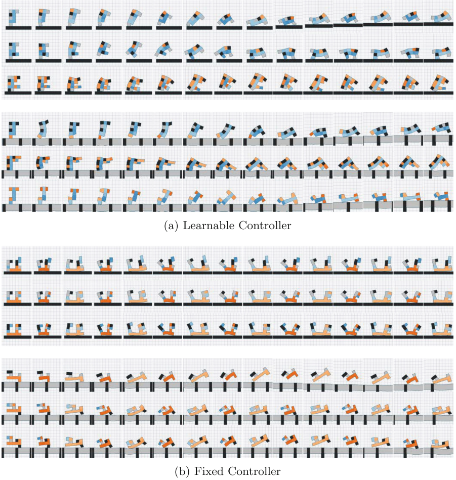
Fig. 4. Timelapse images of three run champions' behavior from each of the two tasks of the (5,5) morphology space, co-optimized brain and body (a) and morphology-only optimization with fixed control (b). Learnable controllers demonstrate more diversity, especially in the Walker-v0 environment. Most of the individuals with learnable controllers (a) find a bipedal (rows 1, 2, 4–6) or monopedal gait (row 3). Fixed controllers (b) show one common behavior on flat ground (rows 1–3), consisting of an active bottom with two vertical apparatus at the front and back, resembling a head and a tail. When the muscle at the bottom of the robot contracts, vertical apparatuses help the bottom part form an arch, creating front and back legs to locomote. In the bridge environment (rows 4–6) often includes a thin, horizontal body with active materials, a forward apparatus resembling a leg, and some upper body (presumably used for balancing). Individuals with this body plan throw themselves forward by actuating their muscles in phase and pulling themselves forward with their forward apparatus, achieving bipedal locomotion.
