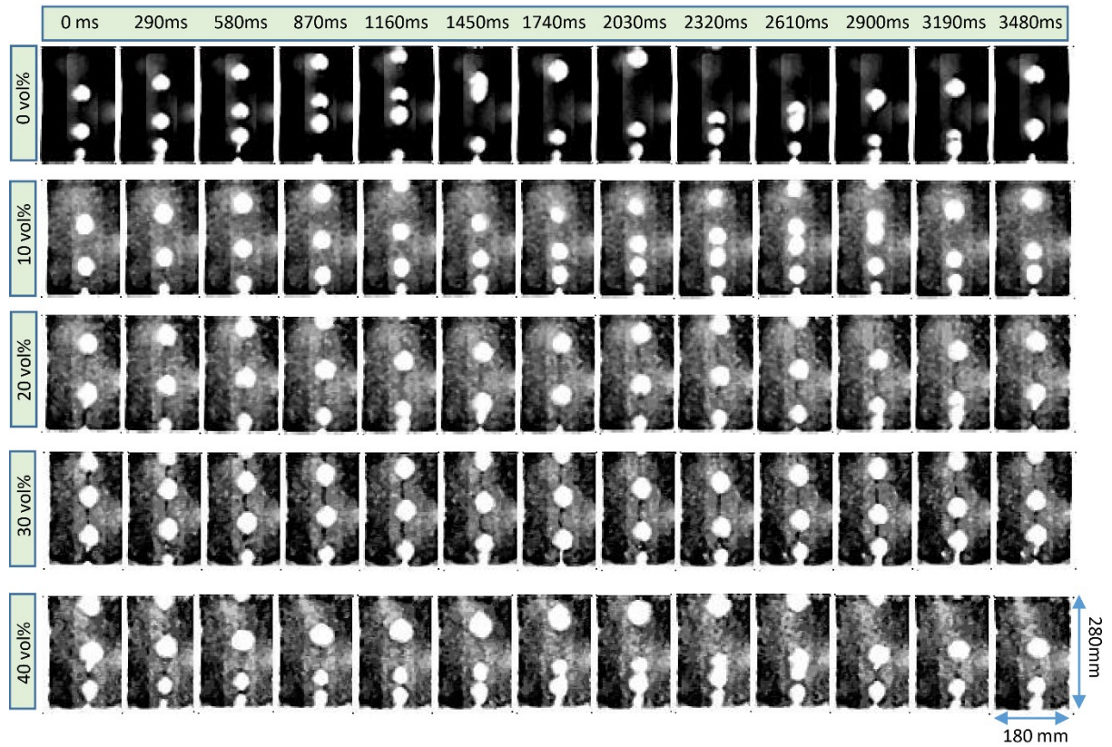
Fig. 5 Time series of 2D central vertical slice images of bubble streams rising through suspensions with different volume fractions. Injection time: 160 ms; idle time: 700 ms. The timestamps are relative to the zero frame chosen for each case; the absolute times of the first tile on each row are 30.3 s, 20.2 s, 5.9 s, 50.3 s, and 80.6 s, respectively.
