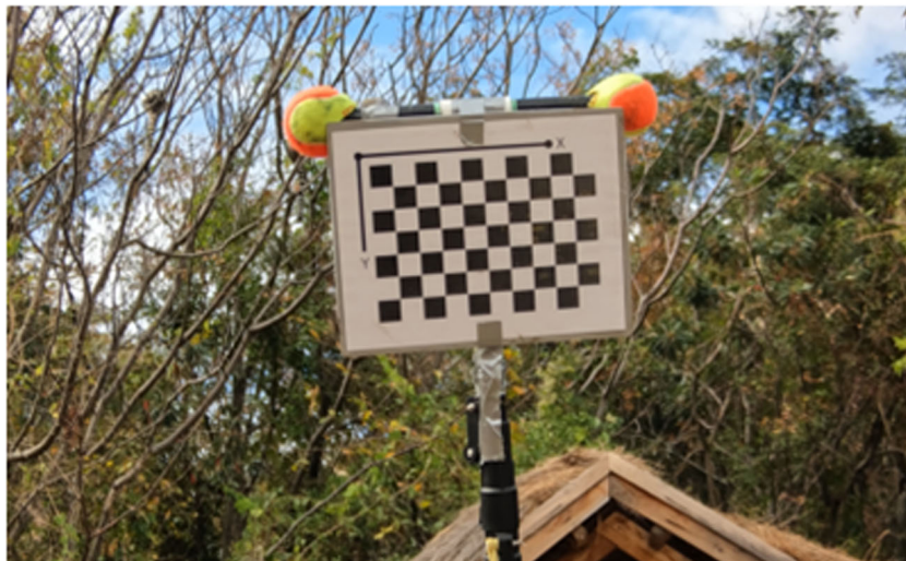
FIGURE 2 Calibration tools. Checkerboard and wand attached to the 10-m pole. For intrinsic calibration the checkerboard faces the cameras; for extrinsic calibrations, we rotated the frame such that only the two wand balls are visible to the cameras.
