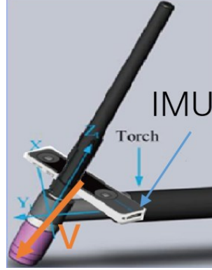
Figure 4 Correlation between sensor coordinate system and endpoint of the bypass electrode.
