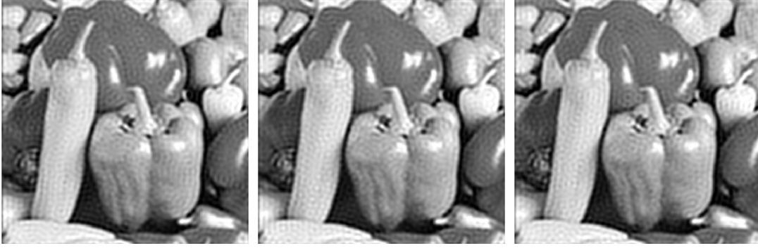
Figure 6. The restoration of images in Figure 4 using a truncated solution with k = 6500 points for gaussian , poisson and salt&pepper noise, left to right plots respectively. The relative errors for these images are 0.0914, 0.0918 and 0.0917, rounded to 3 significant digits. This compares with the optimal errors obtained for these images for the blue vertical lines indicated in the Picard plots in Figure 5 , 0.0911, 0.0914, and 0.0912, respectively.
