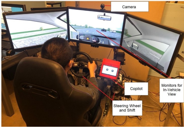
Fig. 2: The cooperative driving testbed setup.
