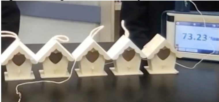
Figure 2. Testing albedo of different paint combinations to lower temperature
