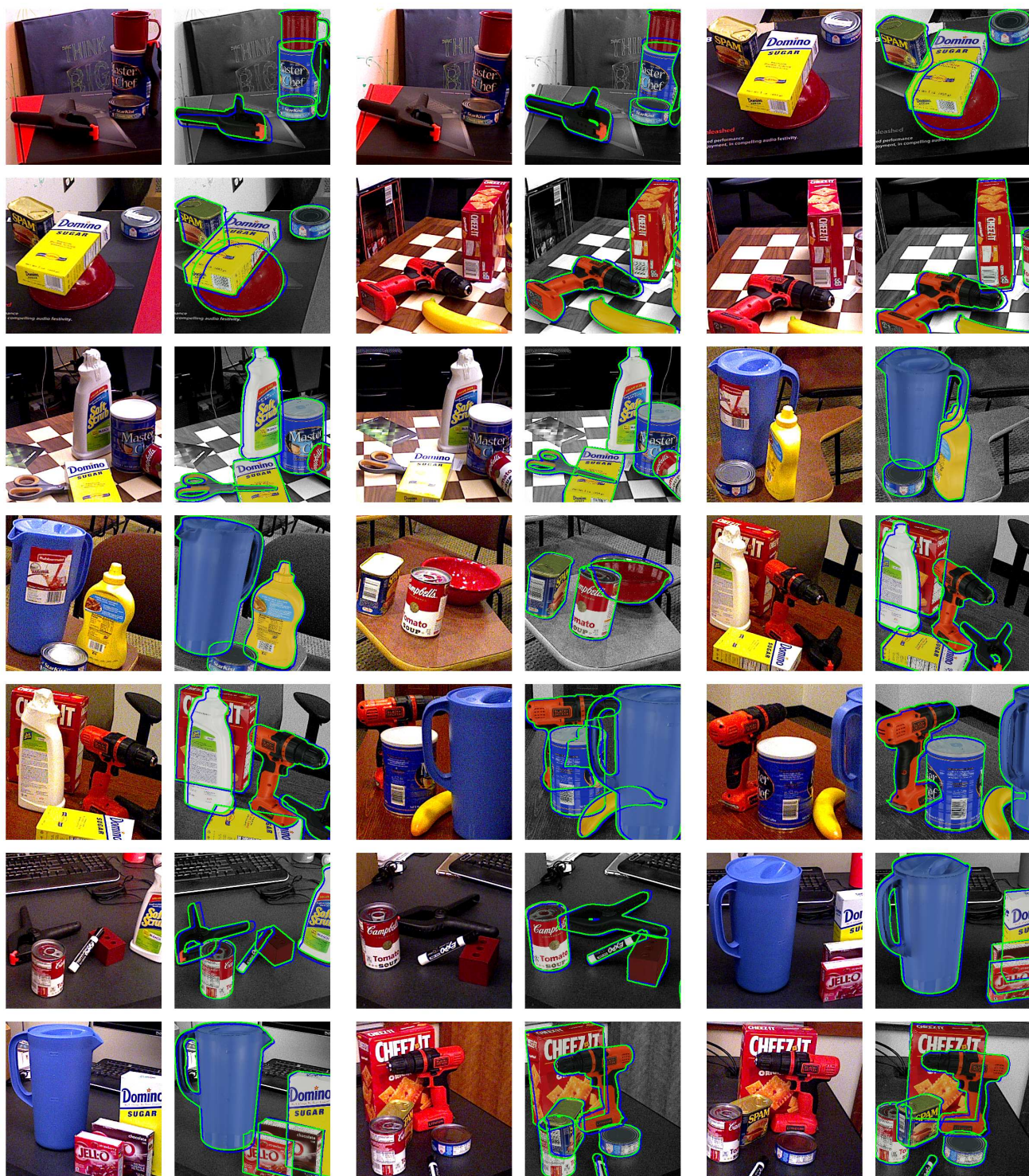
Figure 7: Qualitative results on the YCB-V dataset. For each image on the left, we visualize the 6D pose by rendering the 3D CAD models and highlighting the contours on the right. Blue color denotes ground truth and green color denotes the prediction from CheckerPose.
