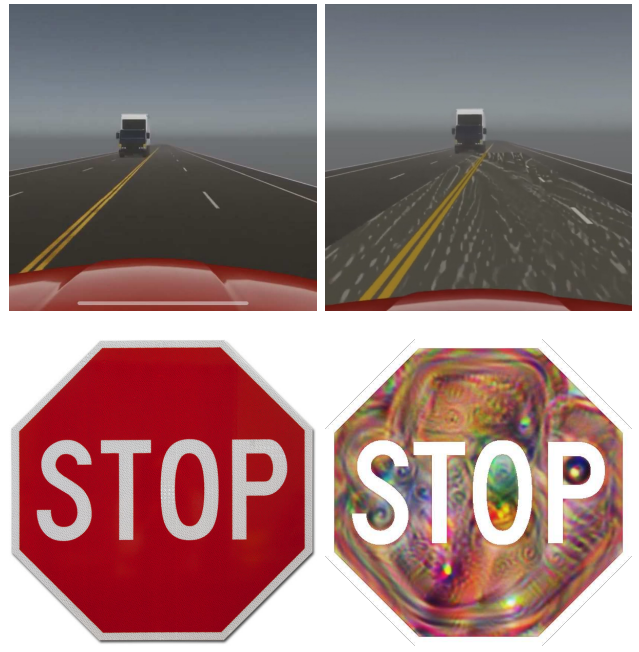
Fig. 1: Images for object detection and autonomous driving projection. Top row shows images for road-surface scenario and bottom row shows images for stop-sign scenario. Left column shows the benign images and right column shows the adversarial images.
