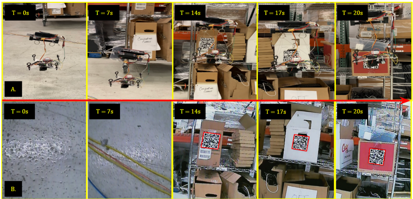
Figure 8: CDPR traveling through the warehouse, moving inline with storage racks, and scanning inventory. Top section A shows the CDPR's scanning path and bottom section B shows the camera's POV
