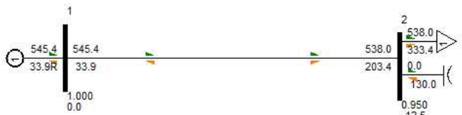
Fig. 3. Power flow for adding a 144 MVAR shunt capacitor at bus 2 to feed 538 MW at V_2 = 0.95 p.u.
