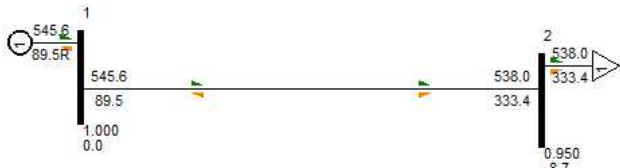
Fig. 5. Power flow for 538 MW with \cos \theta = 0.85 at V_2 = 0.95 p.u. through a line with optimized parameters.
