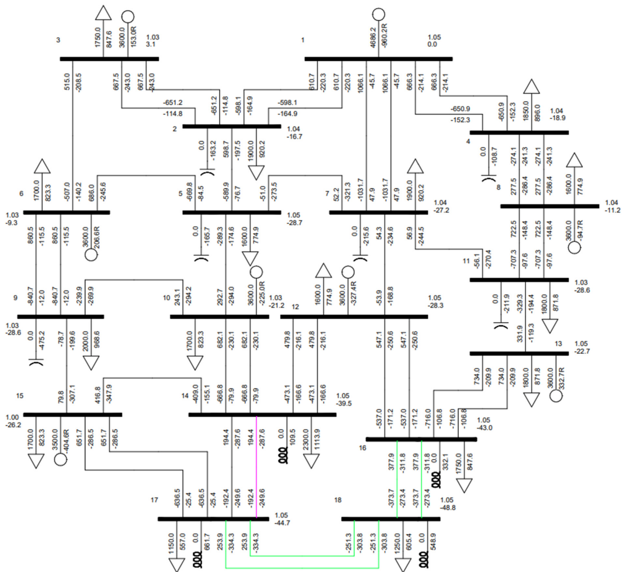
Figure 3. TEP with the unconventional HSIL line (green) and conventional line (purple).
