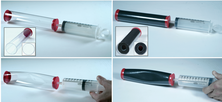
Figure 1. A teaching model illustrates buckling in cylindrical shells. Left: a thin shell (undeformed in the upper part, 40 mm in diameter, 0.4 mm wall thickness made up of plastic) buckles under external pressure when air is extracted from it (lower part), resulting in ovalization. Right: buckling is also induced in a cylindrical shell with an inner core (a tubular rubber foam); in this experiment, the core's stiffness is insufficient to induce bifurcation in a small-wavelength mode, so that in both cases ovalization occurs. Note the position of the plunger inside the syringe showing that the pressure load is higher in the experiment with the internal core.
