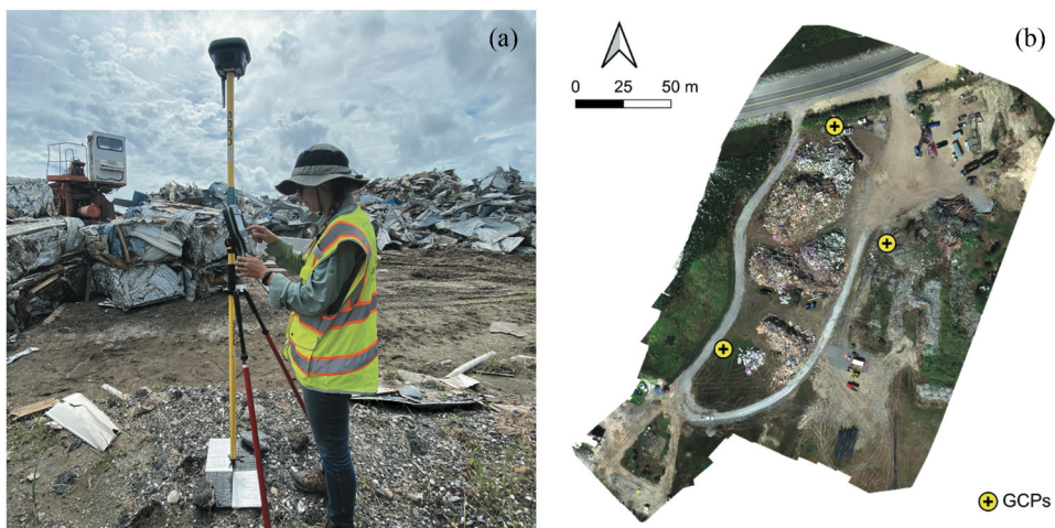
Figure 2. UAV data collection: (a) GCP surveying; and (b) their locations.
