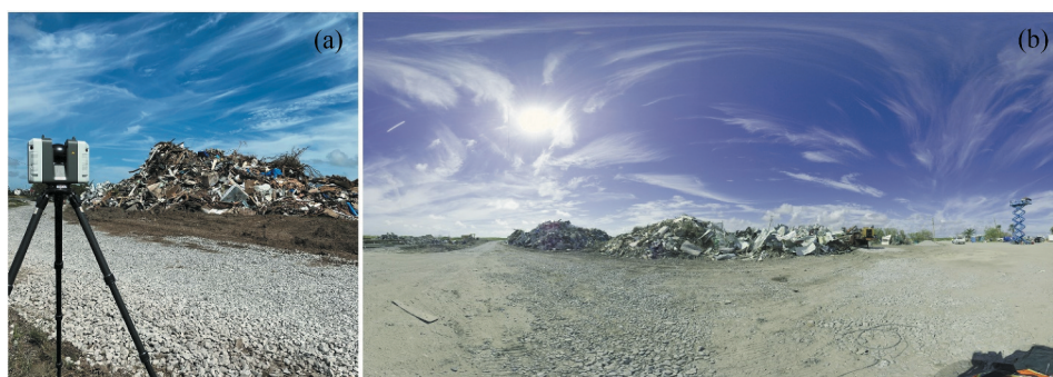
Figure 3. TLS data collection: (a) TLS during scan; and (b) image of site captured via TLS.
