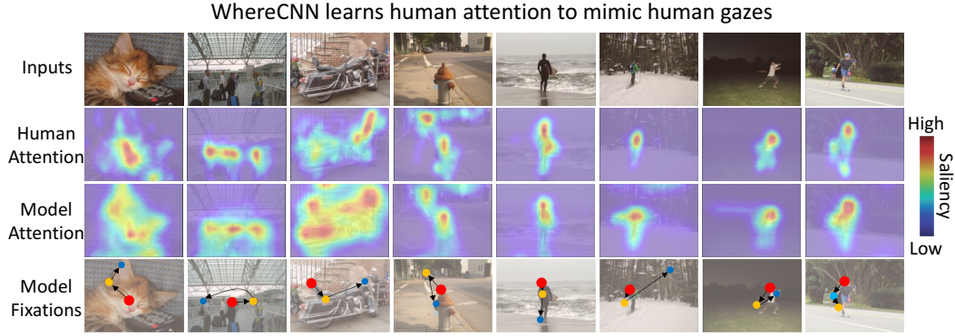
Figure 2: Saliency prediction. Given an image (1st row), WhereCNN generates a saliency map (3rd row) similar to the map of human attention (2nd row). Sampling this saliency map generates a sequence of fixations (as red/orange/blue circles in the order of time in the 4th row) similar to human saccadic eye movements (not shown).
