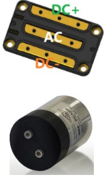
Fig. 1. The schematic of the single-phase ANPC with two CCLs labeled in dashed lines and color labeled parasitic inductance of each component with the pictures of the SiC power module and cylinder DC link capacitor used for the design.
