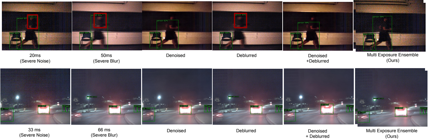
Fig. 9: Object Detection Results on Real Captures: Scene in the first row contains an indoor scenario with two objects: a person (moving) and a chair (stationary). Single Exposures are severely affected by noise and/or blur: detects false positives or inaccurate bounding boxes. Scene in the second row contains a driving scenario with a car (moving) on the left and traffic light (stationary) in the front. Single Exposures fail to detect the moving car or the stationary traffic light. Multi-Exposure Ensemble approach (right) leverages multiple exposures and detects all objects with correct labels and tight bounding boxes in both scenes.
