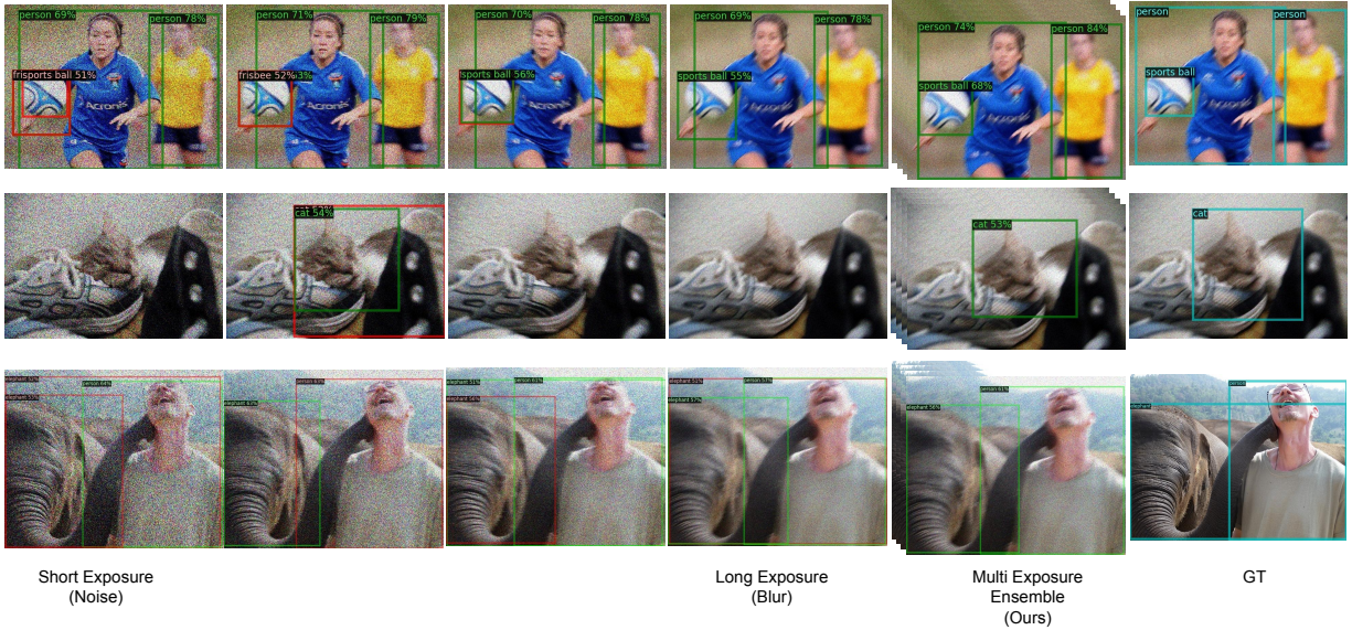
Fig. 10: Object Detection Results on MS-COCO dataset: Correct/Incorrect predictions are highlighted with green/red and ground truth boxes are highlighted with blue in the clean image. Single Exposures have a lot more false positives (red) while our approach effectively removes those cases. For the first scene, our approach produces tighter bounding boxes than individual predictions (Better viewed on screen).
