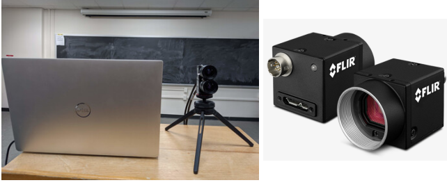
Fig. 7: Camera Setup for capturing multiple exposure images
