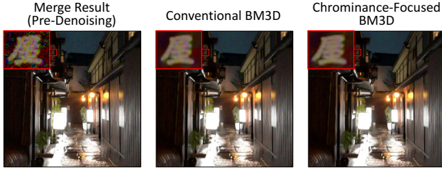
Fig. 6. Denoising with chrominance-focused BM3D. By applying different level of denoising to the luminance and chrominance channels, chrominance-focused BM3D is able to suppress the color noise while maintain more structural details in the luminance channel.
