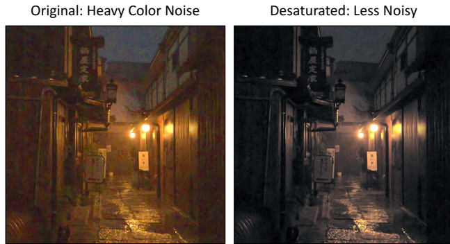
Fig. 20. Noise-aware visualization. (Left) The original image contains significant color noise due to low light. (Right) The proposed noise-aware visualization reduces saturation of the dark pixels and suppresses noise.
