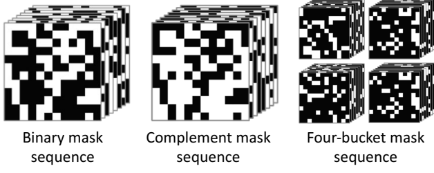
Figure 3: Modulating masks for video compressive sensing. (left) A single VCS measurement temporally compresses a sequence of frames using binary random masks. (center) Two-bucket cameras capture an additional measurement by using the complementary mask sequence. (right) We propose using multi-bucket captures by randomly choosing an active bucket for each frame. Both two-bucket and multi-bucket captures have 100% light efficiency. All masks are visualized here for 16 \times 16 pixels.
