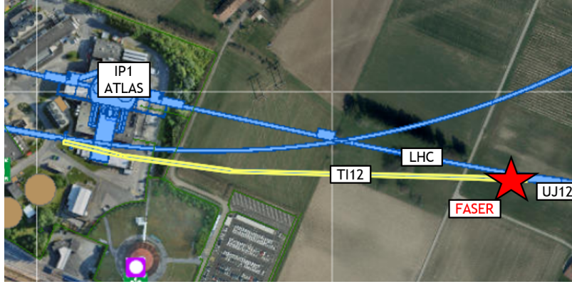
Figure 1. The FASER location: TI12 tunnel, 480 m downstream of the ATLAS interaction point. The detector is located along the beam collision axis line-of-sight.
