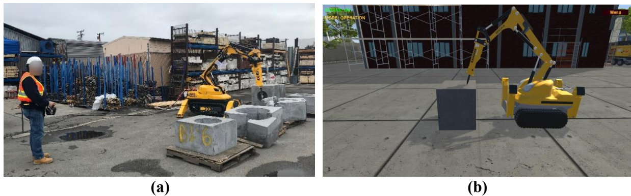
Figure 1. (a) Remotely operated Brokk 110 and (b) teleoperated Brokk 110 (3D model).
