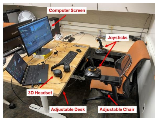
Figure 2. Proposed teleoperation workstation.
